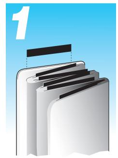
Locate *Six Panel Base* section (footed chanels on bottom). Stand on feet and fold panels to form an accordian or zig zag effect. *Insert stacking guides* into grooves in top of base panels.
