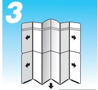
Unfold panels. Push center hinge forward and slide side panels forward so that the eight panel arch-top center section forms a recessed area for header.
