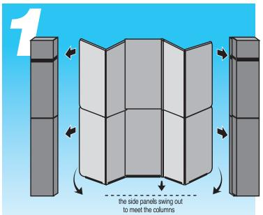
After assembling the columns,see column assembly sheet.
