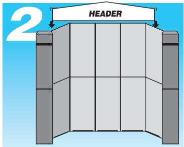
Place the Header Graphics on the header frame then attach the complete Header onto the finished Unit—see header graphics application sheet—This will aid in stability of the center section, and ensure proper spacing of panels. Note the header fits flush with front of columns
