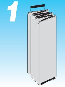
Locate *Five panel Base* section (footed charnels on bottom). Stand on feet and fold panels to form an accordion or zig zag effect. *Insert stacking guides* into groves in top of base panels. Fold matching *FivePanel Top* section as above and lower onto base. The stacking guides insure proper alignment of upper and lower panels.
