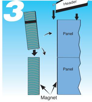
Now, place the top column onto the bottom column. The **square pins** in the lower end of the top column section fit **into** the **square channels** in the bottom column section. After the panel sections are completed, the columns can be **snapped into place** using the **magnets** on the sides of both column and panels.
